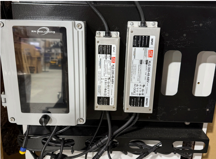
MeanWell drivers are supplied complete as 100% Plug 'N Play – requiring only 1 × 13A CCE plug per driver set.
