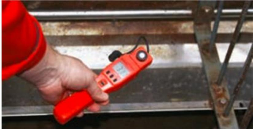
When the light is placed right above the sow, it gives the opportunity to limit the number of lamps in the ceiling, as they are only to be used when there are staff/workers in the stable. Rune Nielsen is turning off the ceiling light and turns on the LED light above the sows, and then he does the same measure as earlier, and now there is more than 300 lux.
